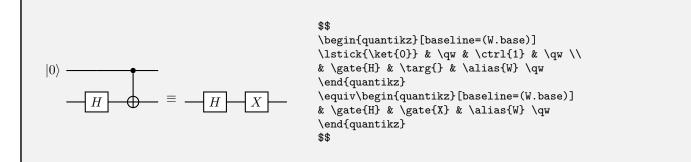
This has aligned the bottom wire of the first circuit with the wire in the second circuit, making the correspondence more obvious. However, the  $\equiv$  sign is now in the wrong place, with its baseline placed at the same point as the baseline of the circuits. We can fix this with a vertical shift of the two diagrams. We demonstrate two different ways of achieving the same effect (the only important feature is that both diagrams have the same shift).
