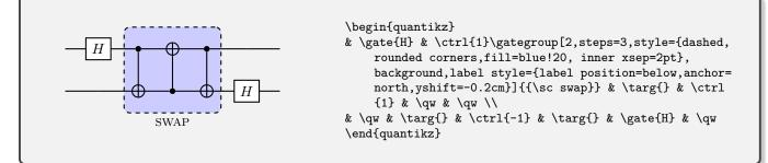
Note that it is often good to use anchor=mid for label anchors because if you have multiple labels, this will help get them horizontally aligned. It just means you have to use some yshift to move the label off the border around the gategroup.
