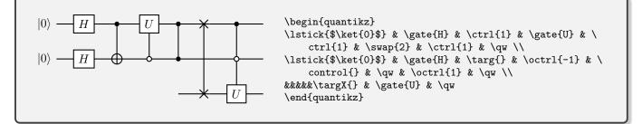
If you want a gate that is one control and several targets, you may need the command  $vqw{1}$  (vertical quantum wire) to create vertical connections, or possibly  $vcw{1}$  to create the classical version.
