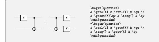
If you cannot identify the offending gate, and particularly if the operation is not a standard \gate command, you might be better off combining the two circuits in a single circuit with no wires joining the two parts. The spacing works better if your circuit has an odd number of wires, otherwise you have to add an extra row in the middle, and then change the spacing of that row with its neighbours.
