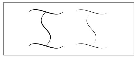
With a copperplate pen, the segments of a path are tapered. Copperplate and normal pens can be mixed. Any part of the pen specification that has no length is treated as a copperplate pen.
