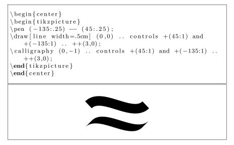
The paths are identical in definition but the first is drawn using the standard TikZ path with a line width of .5cm. The second is "stroked" with a calligraphic pen of width .5cm angled at 45 degrees.
