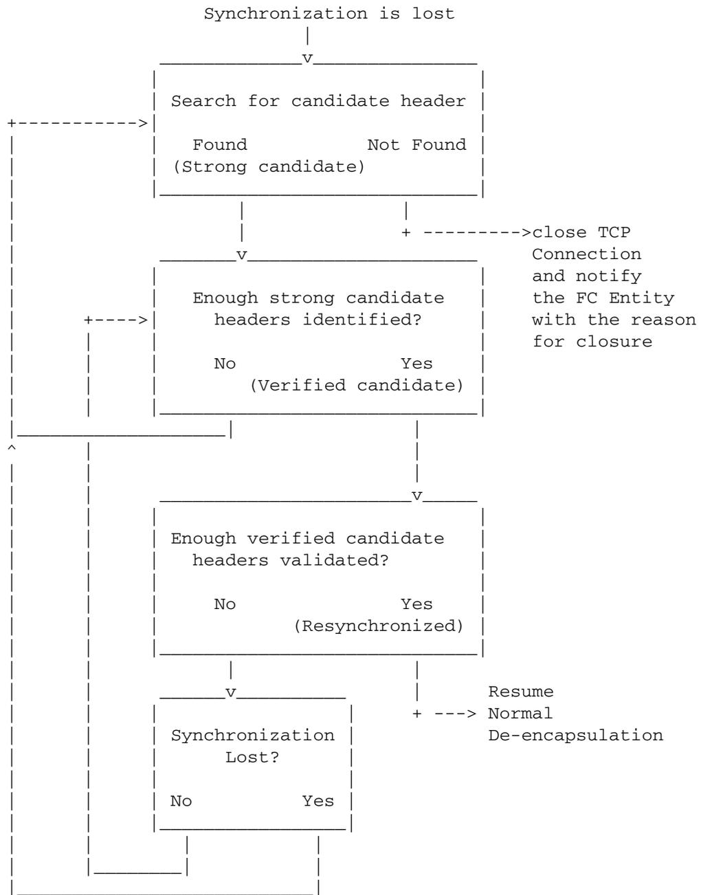
Fig. 15 Flow diagram of simple synchronization example
